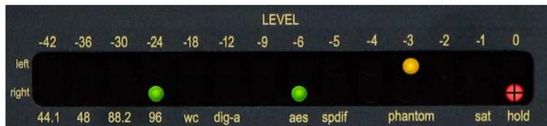
96kHz SF, AES output format, phantom power enabled left channel, meter peak hold “off”
